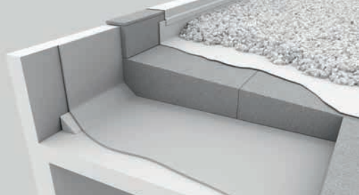
Flat roof insulation
